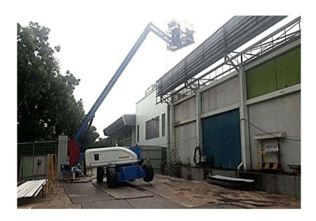
I shall refer to this photograph as the tilting incident photograph. It shows the Boom Lift after it had shut off and before the workers were rescued. Only the upper boom had been deployed. It had been elevated to an angle of about 45 to 50 degrees. One wheel had lost contact with the ground.
